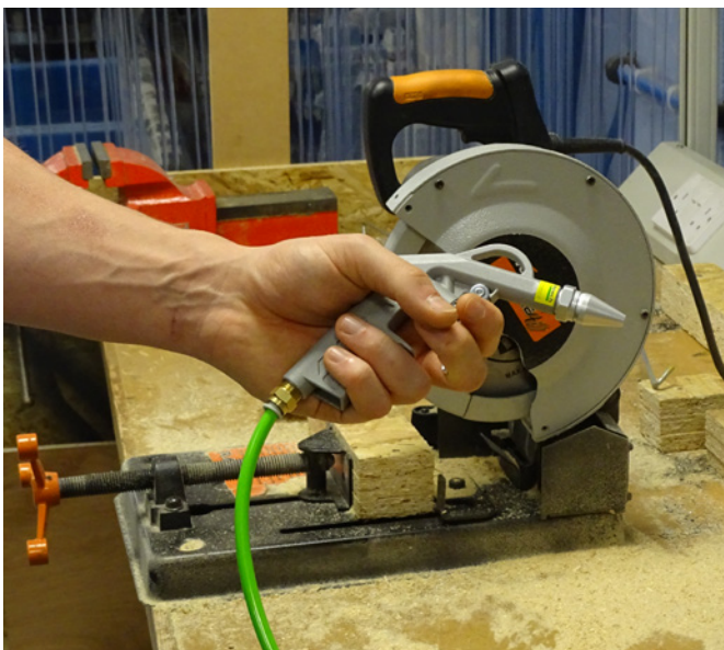
Blowgun used to blow swarf from work station.
